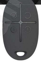
The SpaceControl from Ajax Systems is a key fob for controlling security modes. Features a panic button for sending alarms to your inner circle and a security company in case of trouble.
