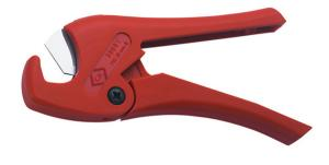
Features & Benefits  $\sim$  Glass fibre reinforced polycarbonate body  $\sim$  Razor sharp stainless steel blade for efficient cutting of: PVC conduit, blue water mains, plastic pipe, rubber hose, pneumatic pipe, electrical sleeving, etc.  $\sim$  Capacity: 28 mm  $\sim$  Total Length: 195 mm
